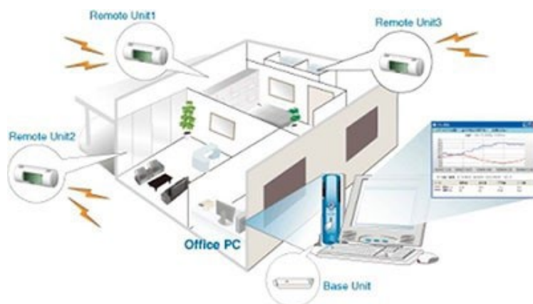
Figure 3: Networked System in an Office
