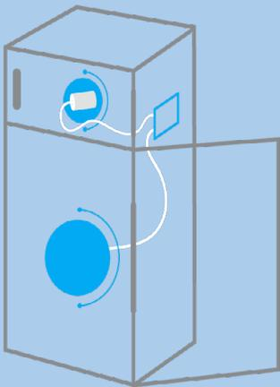
The position of the probe in the storage cavity is important, as it measures the temperature at a single point in space. That point should be where it best reflects the temperatures of the material in the refrigerator or freezer. If the refrigerator cools by forced air, having the probe in the airflow will yield more fluctuations than if it is in a still area of the refrigerator.
